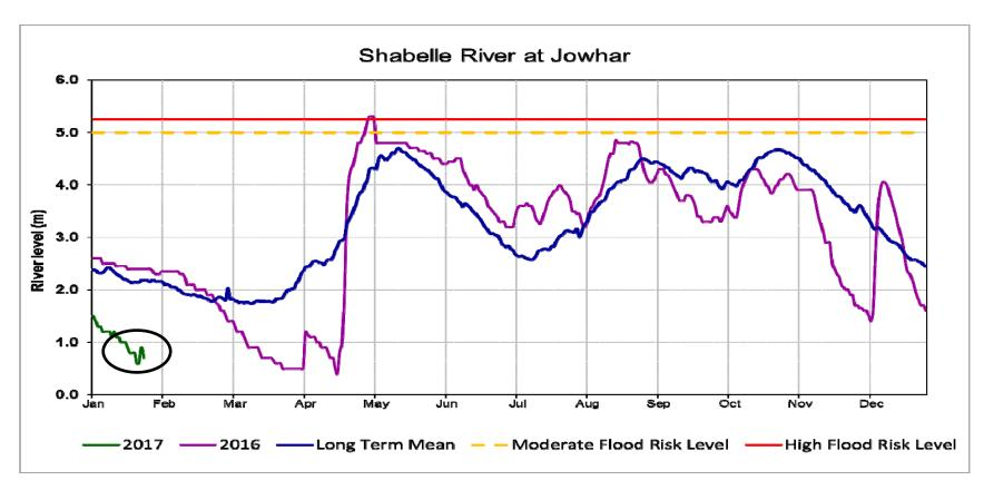
River levels at Jowhar (Middle reach) has reached historical minimum which was also reached in March 2016. The dry river bed level is at 0.5m which has been significantly raised by sedimentation over the years.
