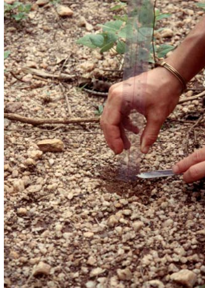
Figure 3.14 - Measuring the armour layer with a ruler (Stocking & Murnaghan, 2000)
