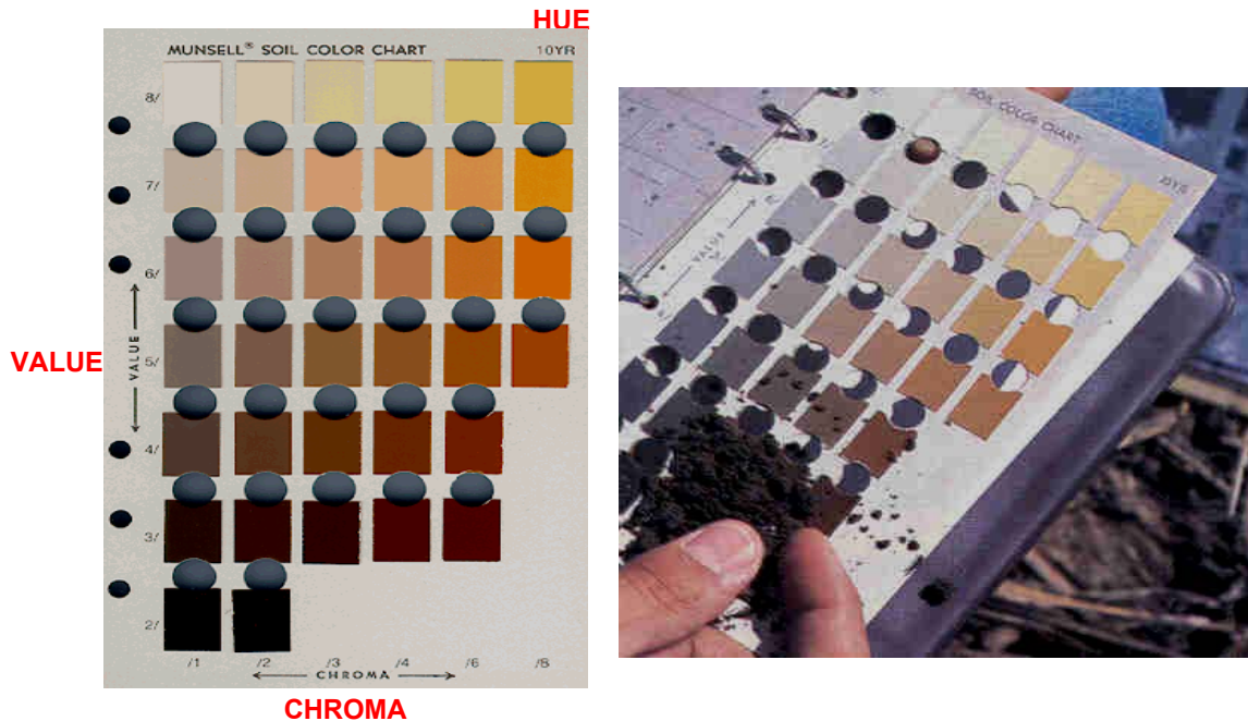
Figure 2.4 - Munsell Soil Colour Chart and an example of how to use it
