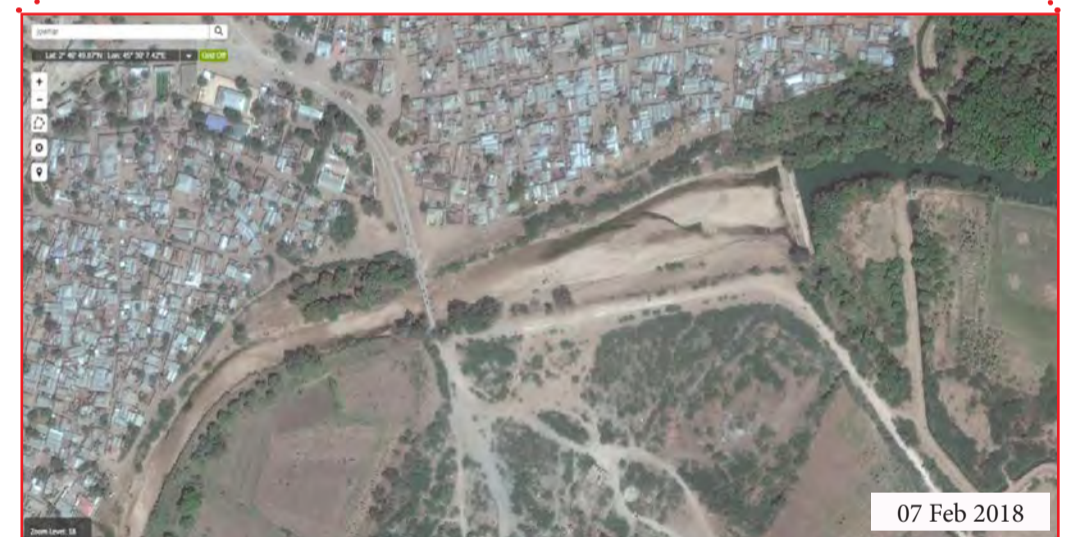
The image shows the weir in Jowhar. Downstream of the weir the river is dry as evidenced by the outcropping of the river bed. The two canals upstream the weir are active as they are providing water to the surrounding irrigated area. However, the amount of irrigated land is confined just along the primary canal, as shown with yellow outlined circles in the image showing the overview of the area. It is also noted that the majority of fields irrigated by the canals downstream the weir are not cropped.
