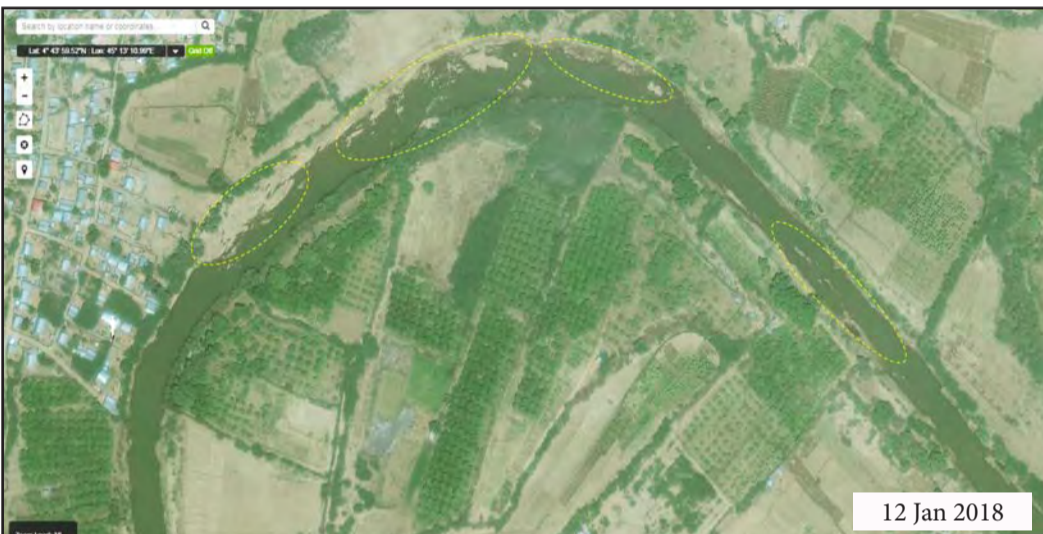
The image shows that river level is very low, as evidenced by the presence of sand deposits/river bed (yellow outlined) occurring along the river.
